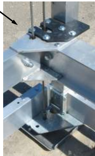
Kitty corner to winch column area assembled view
